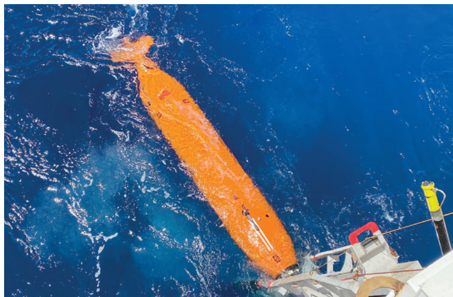
Autonomous Underwater Vehicles (AUVs) carry a variety of equipment for sampling and surveying such as cameras, sonars and depth sensors, which help to indicate nodule locations
