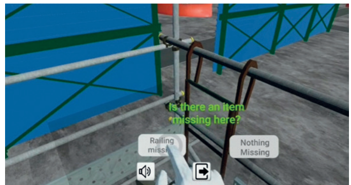
The AR learning aid for the four-stroke engine sequence (L) and VR simulation of scenario-based safety decision making (R) provide trainees with an immersive learning experience
